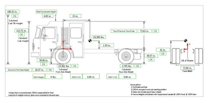
Calculated Apparatus Weight19,306 lbs.Calculated Apparatus Z-CG33 in.Calculated Apparatus Y-CG1.55 in.
